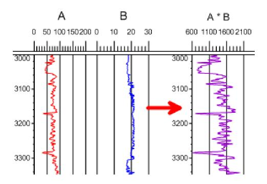
Apply mathematical functions to existing logs to create new logs
