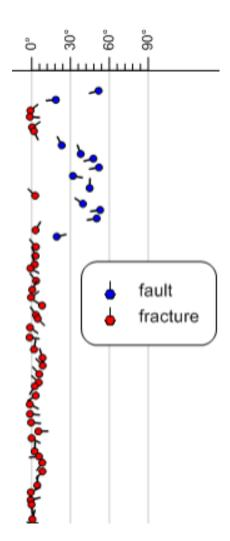
Display dip and dip direction measurements using a tadpole log.
